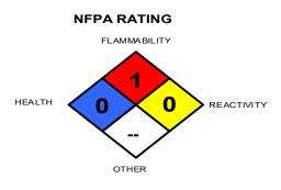
Hazard Scale: 0 = Minimal 1 = Slight 2 = Moderate 3 = Serious 4 = Severe
