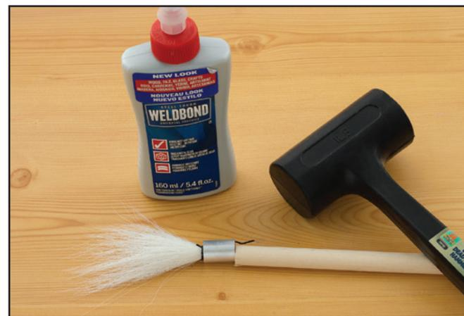
**Step 3:** Glue the bristle bundle into the metal tube. Flatten the end of the metal tube nearest the bristles with a mallet.
