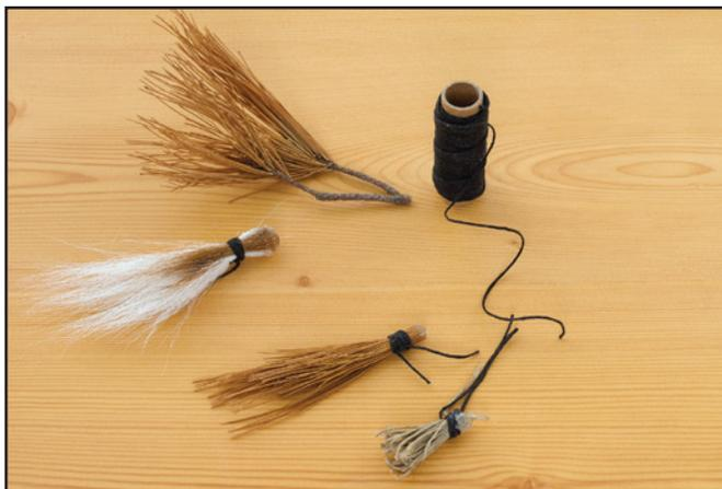
**Step 1:** Using waxed linen thread, tightly tie a bundle of bristles near the base, then dip the end in glue. Allow to dry.
