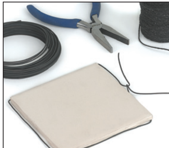
Step 1: Bend annealed wire around a ceramic tile or wood block to make a square shape.
