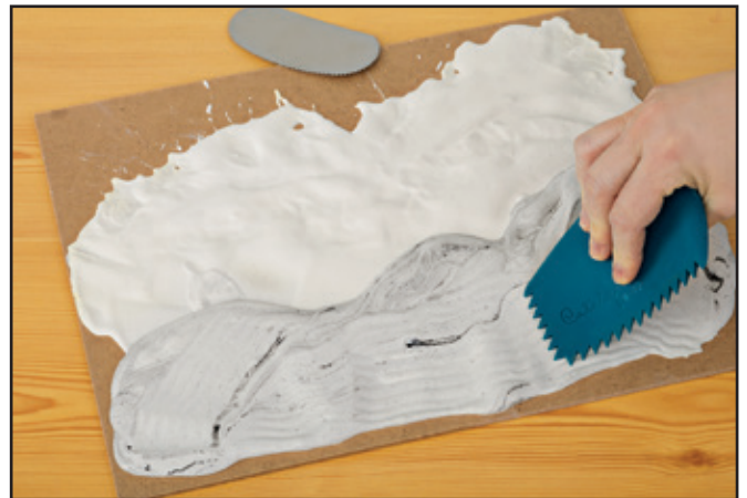
Step 2: Create texture in the plaster by adding inclusions or by applying with toothed scrapers or other tools. Textures can also be impressed when the plaster has set slightly.
