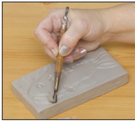
Step 1: Carve into leather-hard clay to create textured mold.
