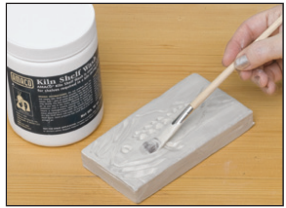
Step 2: After the mold is bisque-fired, apply two thin coats of kiln wash.
