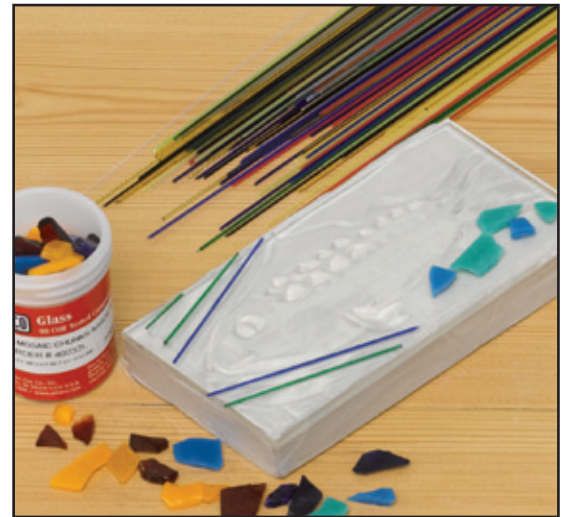
Step 4: Place a sheet of clear glass over the mold. Add glass stringers or mosaic chunks, if desired.
