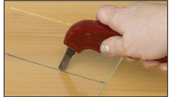
Step 3: Cut clear glass to fit the size of the mold.
