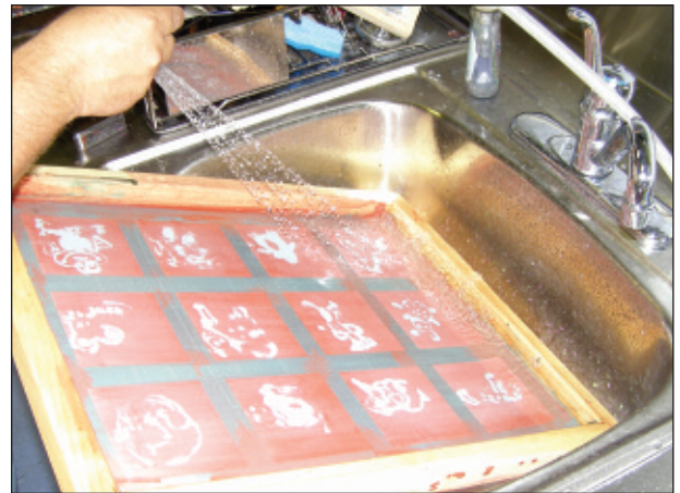
(C) When the screen filler is dry, rinse the screen in cold water
