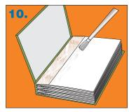
The text block is placed on the inside of the cover blank. The end sheet is glued to the cover. Finally, the book is pressed or clamped between boards and let dry.
