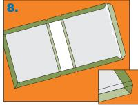
The overhanging book cloth is turned over the covers and spine and glued down with neutral pH adhesive. Corners are mitred using a "bedsheet" tuck.
