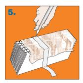
Width dimensions for the cover and spine strip are captured from the text block by wrapping a strip of paper around the spine and marking the spine width and cover size.
